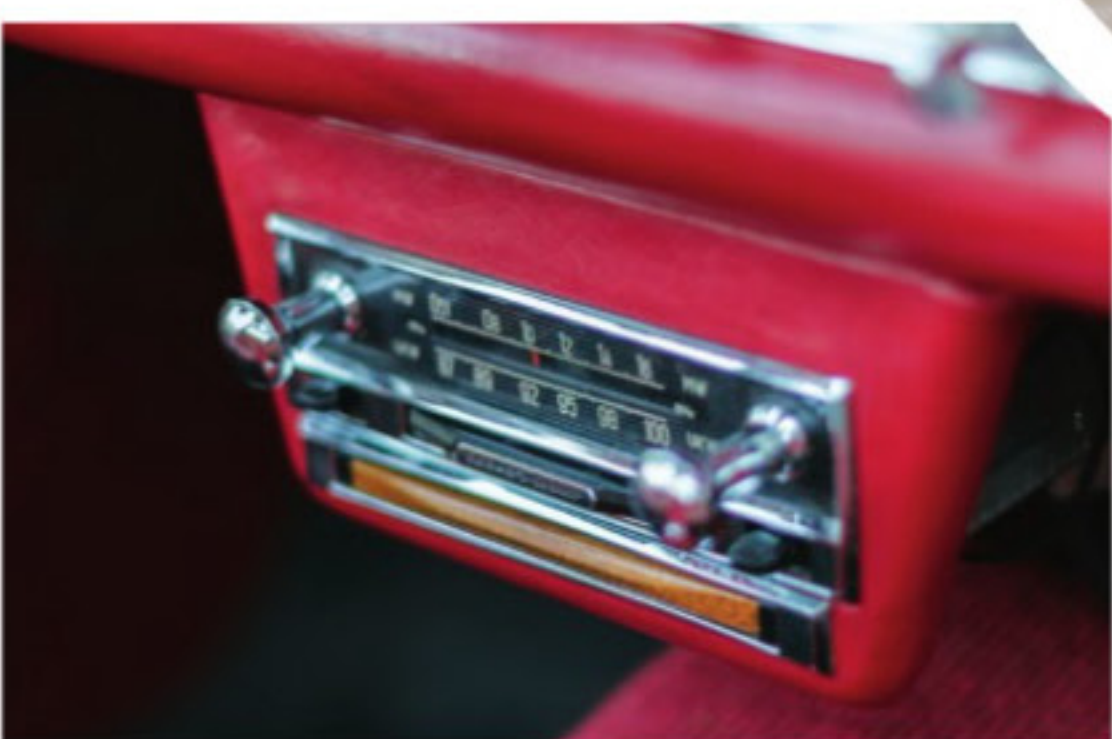
ABOVE A single, streamlined wing mirror adorns the body. ABOVE LEFT Huge air intakes dominate the 300SL's front wings. LEFT Original Becker radio was repaired, and works well.
