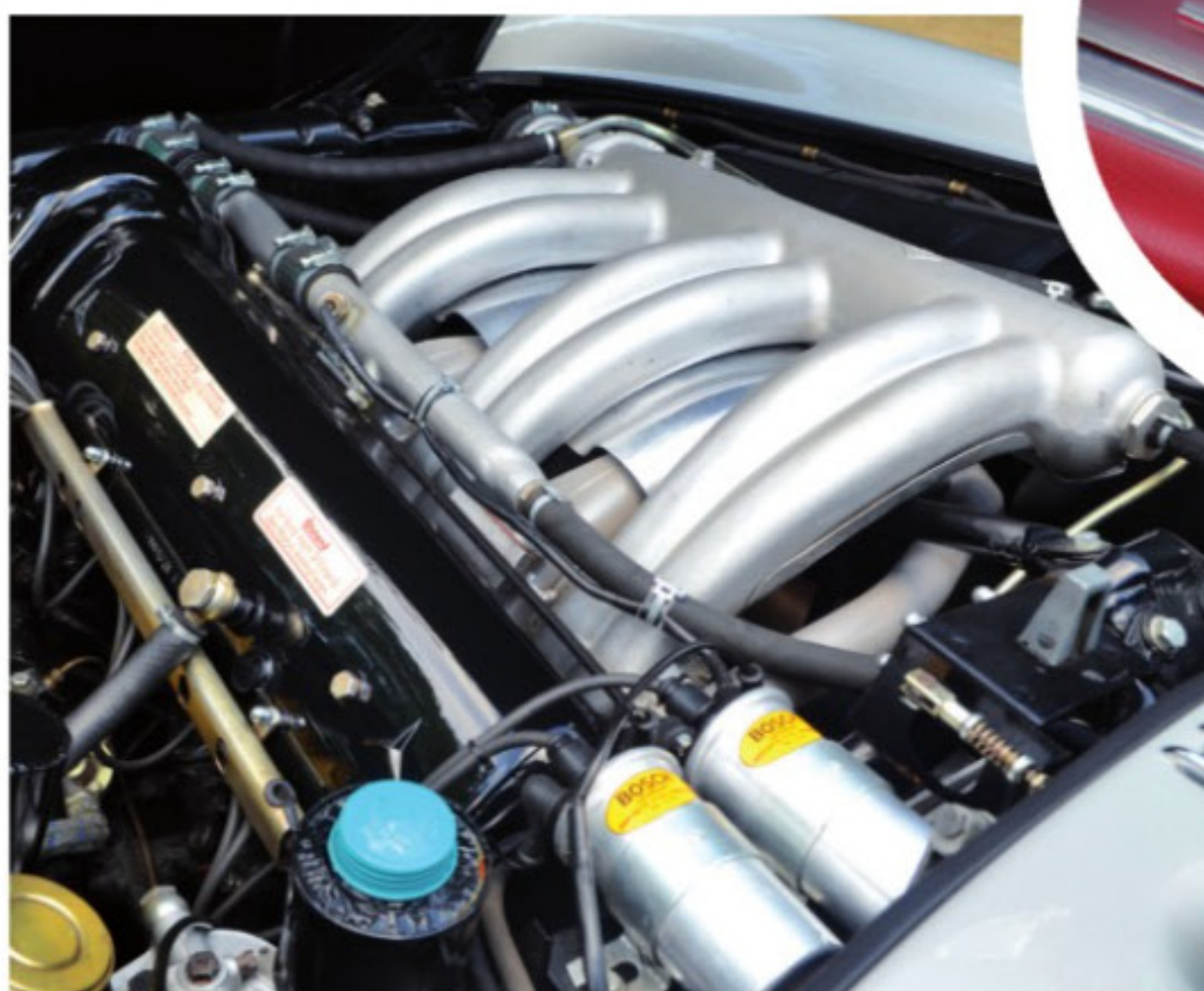
ABOVE Handsome alloy induction tubes feed the M198 six, which produces 212bhp.
