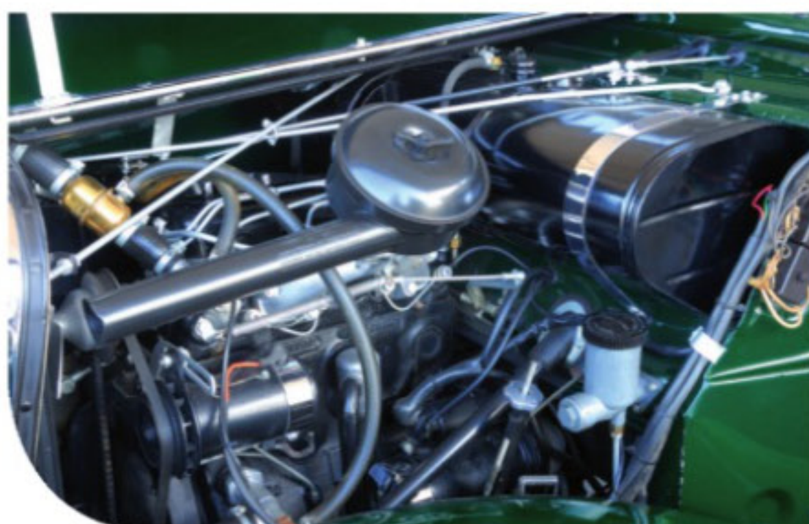
ABOVE Later OM636s modified to cure a running on problem that affected early engines.
